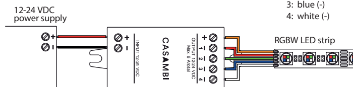
Wiring diagram, RGBW
