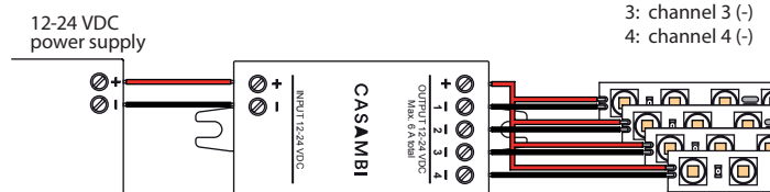
Wiring diagram, 1-4 separate channels
