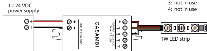
Wiring diagram, tunable white
