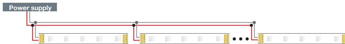
ELECTRICAL CONNECTION: connections in series or parallel
