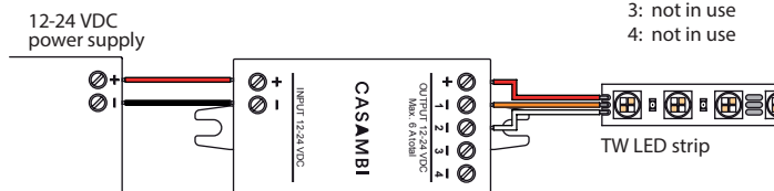
Wiring diagram, 1-4 separate channels
