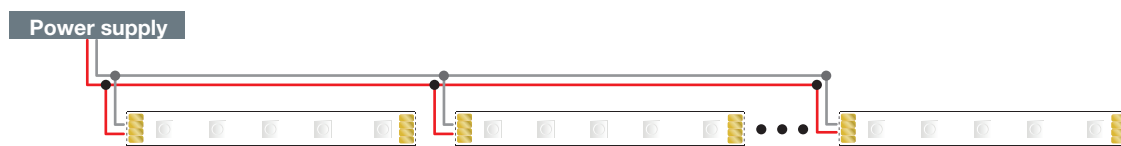
ELECTRICAL CONNECTION: connections in series or parallel
