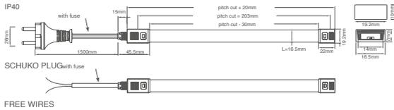
DURASTRIP HiVolt ARCH DIMMABLE - 230V - IP65 Terminal "EX" with Schuko plug or free wires
